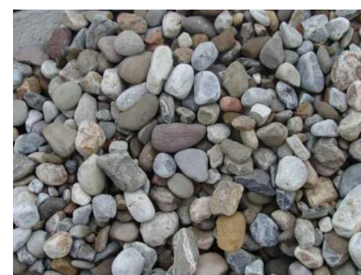
RIVER JACK STONE (1"-3") ON FILTER CLOTH NTS
